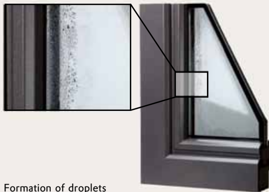
Formation of droplets and a border with the use of silicone oil
